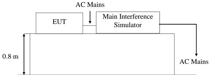
Remark: Combination wave generator and decoupling network are included in test generator.
